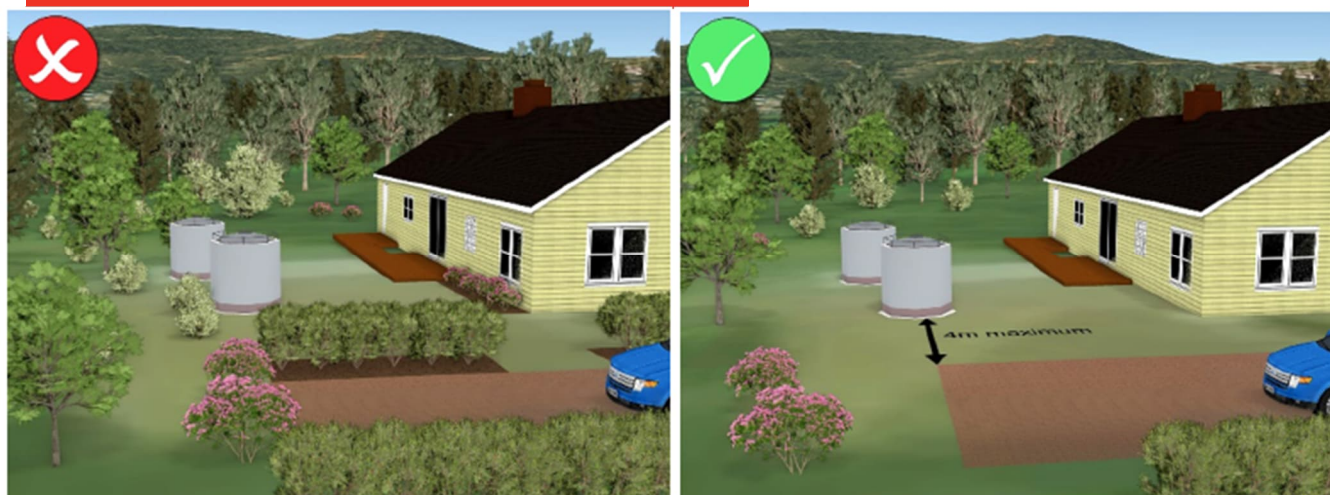
Figure 39 of the Planning for Bushfire Guidelines (Nov 2024): A good and bad example of landscaping around a water tank
