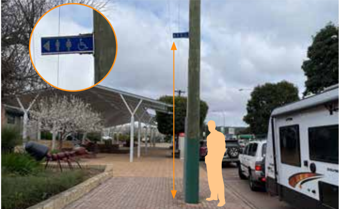
Poor sign placement almost 4m from the ground, too high for most people to even notice
