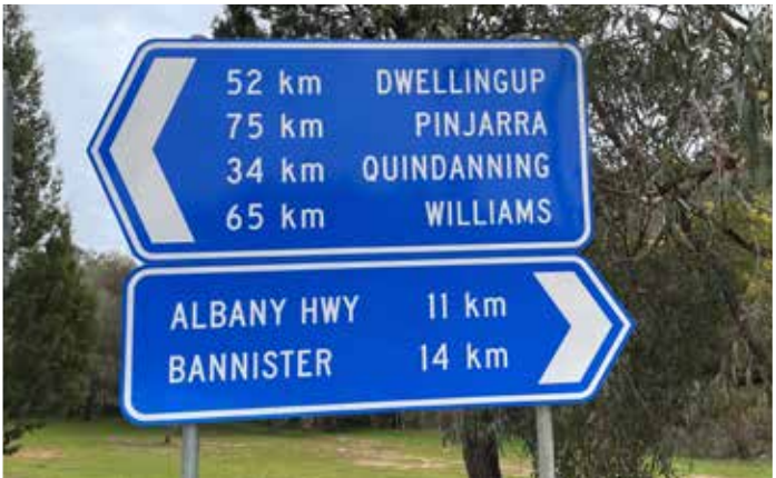
Should be green directional signs - wrong type of sign, wrong location, poor application
