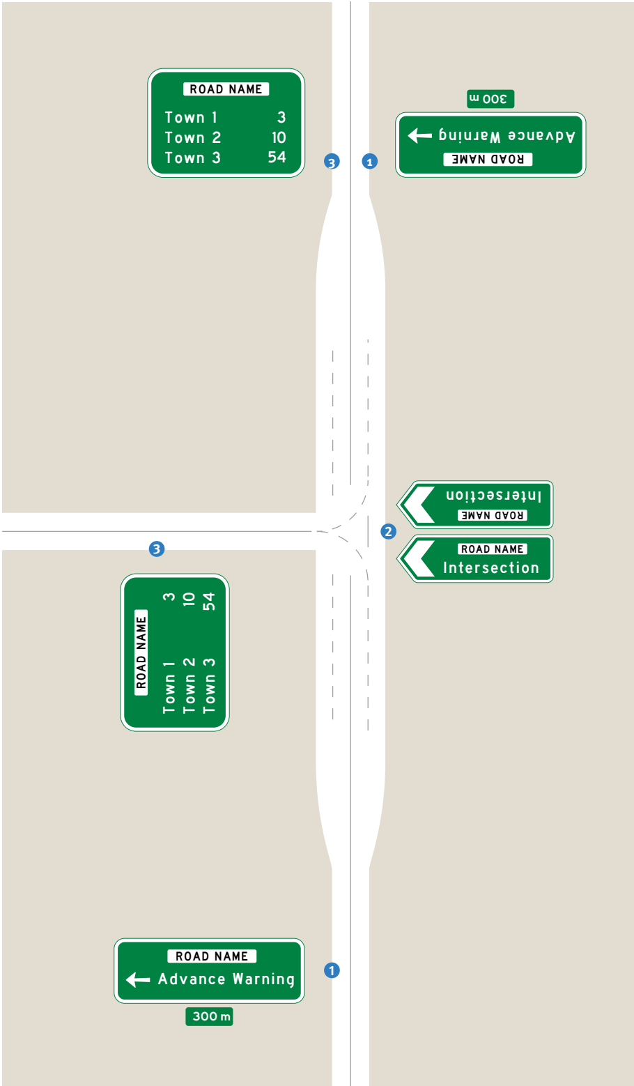
EXAMPLE - Signage placement 1) Advance warning, 2) Intersection 3) Reassurance
